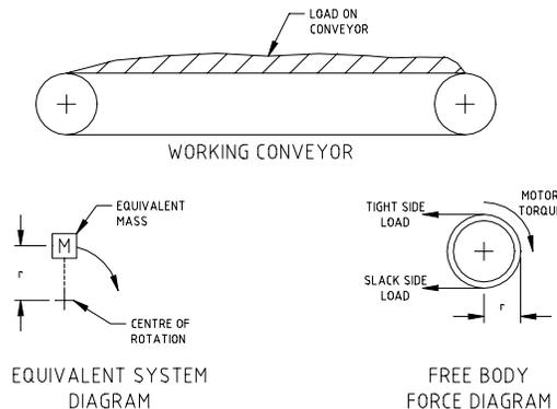
Figure No. 1 Conveyor Inertia
