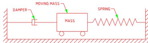
Figure No. 1 A spring-mass damper system.
