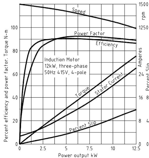
Figure No 1. Electric motor characteristics
