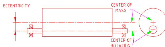
Figure No. 2 Eccentricity between center of mass and center of rotation.
